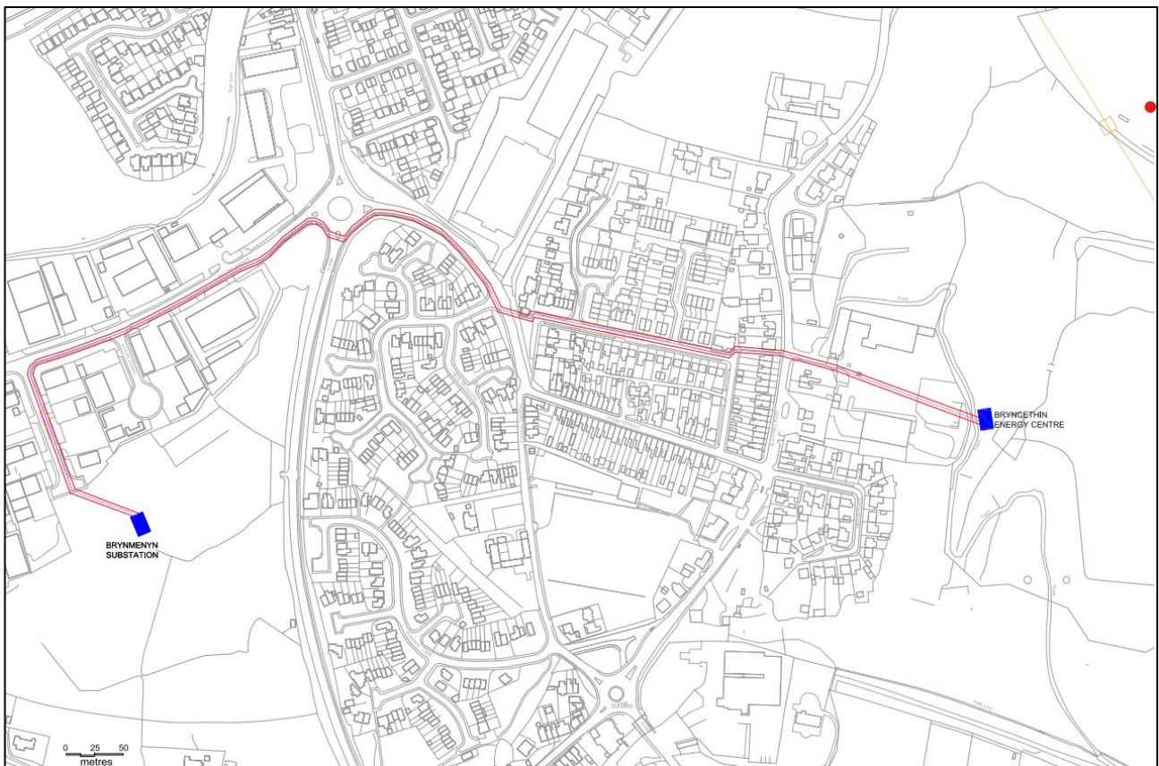
Figure 8: Line of Private Wire Connection
